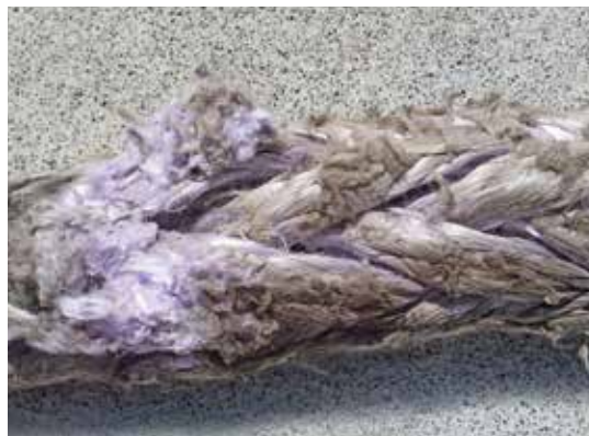
Visual inspection of yarns on rope in this sample shows heavy cutting on two adjacent strands, but only moderate surface abrasion (darker areas on the surface of the strands)
