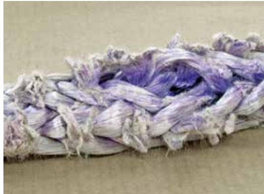
Cut adjacent strands probably caused by rubbing against a sharp corner or edge of metal
