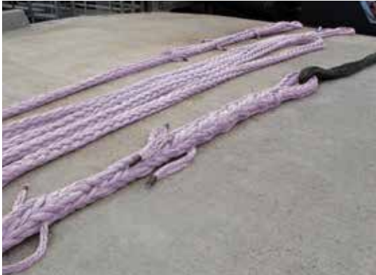
Moran 5/4/3 tuck splice Plasma® 12x12 – which is spectacle-spliced into a pendant. Note exposed “tails” on Moran 5/4/3 splice
