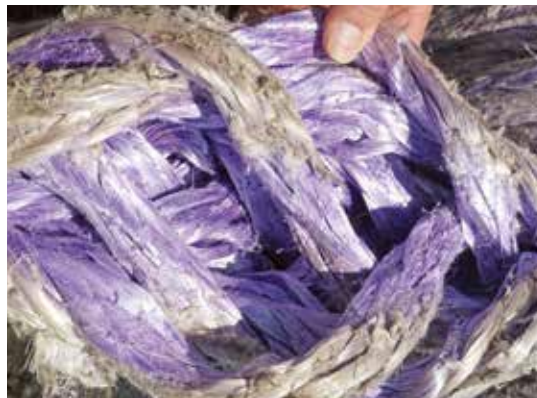
Inspection of hollow core area of Plasma® 12x12 rope. In picture above, no internal wear is observed. Exterior yarn abrasion is noted as "light" and not a problem
