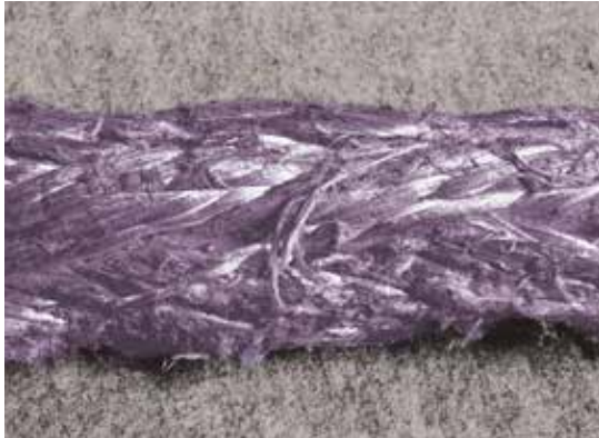
Excessive exterior abrasion wear
