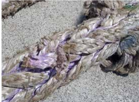
Used piece of Plasma® 12x12 line with abrasion wear on splice area. Note the exposed “tails” which no longer have tape securing the ends. This is an example of a used “floppy” tail
