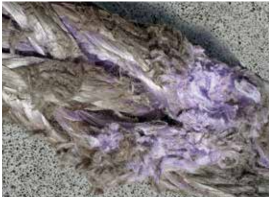
Cut adjacent strands; from its look it may have been cut by a "crossing" wire rope
