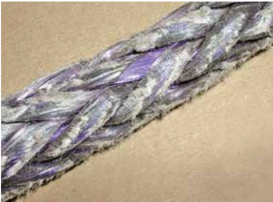
Normal low exterior wear; “fuzziness”
