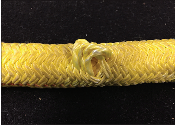
Snagged strands on the jacket; the load bearing core is intact
