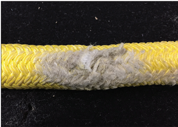
Localized abrasion due to contact with an abrasive surface
