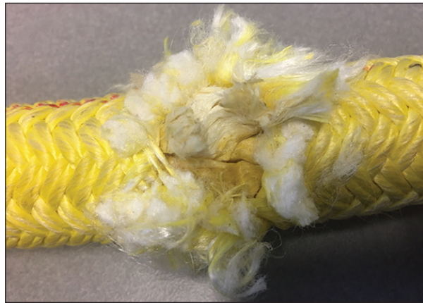
In this case the cut was severe enough to damage the core which results in strength loss
