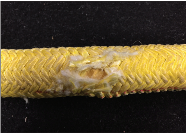
Cut jacket strand; the cut has not damaged the core of the line
