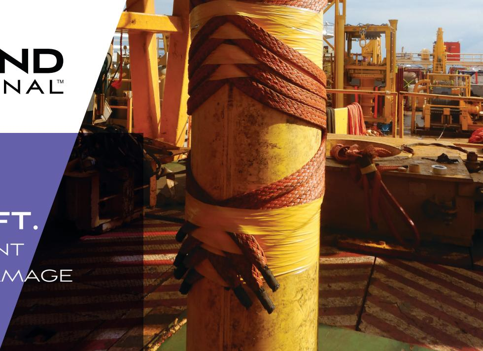
Cortland International Cable Grips (Stoppers) are designed to securely grip a wide range of cables—from large hydraulic umbilicals to small fiber optic cables. They can be used as quick-fit, temporary attachment or tie-off points, or as permanent attachments, depending on application requirements.
