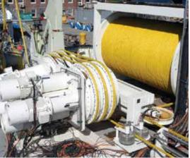
Super Wide Tow Rope Probably the most critical rope within the seismic array, super wide tow ropes need to cope with high levels of tension-tension and cyclic bend fatigue.
