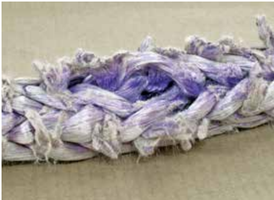
Excessive abrasion wear – volume of total rope in selected area is substantially reduced
