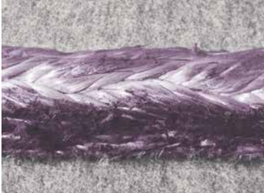
Heavily discolored Plasma® rope from mud, dirt and fluids. Interior is checked to insure no internal yarn damage.
