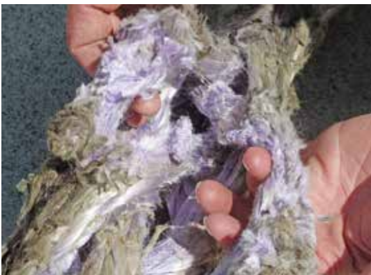
Visual inspection of interior yarns shows wear from abrasion or cutting
