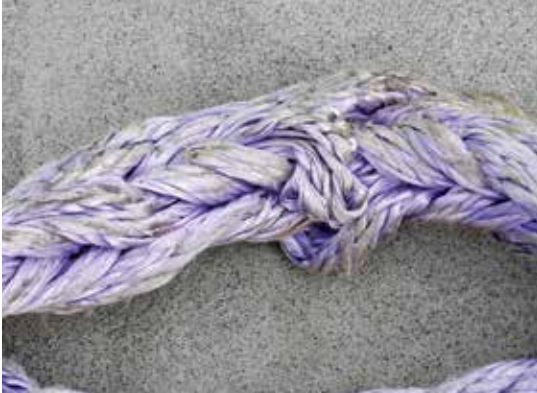
Visual inspection for construction changes, excess twist in rope
