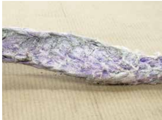
Severe case of compression and construction distortion. Typically this occurs on the bottom layer of a Plasma® winch line compressed against its barrel or flange. If this occurs it is recommended that the severely compressed/ distorted area be cut out before further use.
