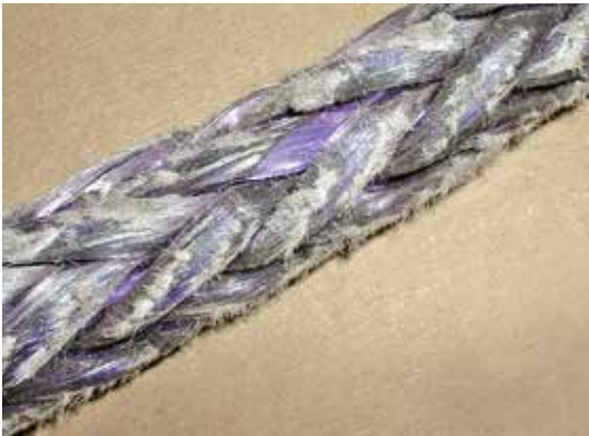
Normal low exterior wear; “fuzziness”
