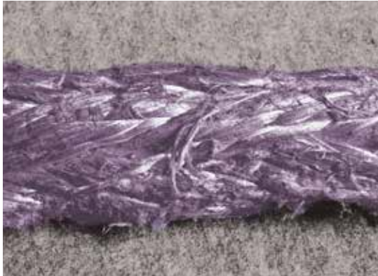
Excessive exterior abrasion wear
