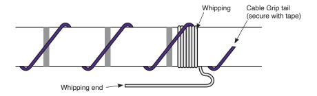
6. Select the second tail (nearest the lower left quadrant, #2) and wrap in the opposite helix direction to the first tail so that the two strands form a symmetrical row of x's along the line of the cable. Whip the first and second tails tightly to the cable and leave the tail end of the whipping cord attached. Trim off excess Cable Grip tail, or tape it to the cable.
