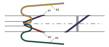
5. Wrap the Cable Grip tail beyond the whipping and secure the end with tape.
