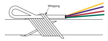
2. Make marks along the cable with a marker or tape bands at these multiples of the cable diameter (8D=8x the cable diameter, 6D=6x cable dia, etc.), beginning at the base of the Cable Grip: 8D, 8D, 6D, 6D, 6D, 6D, 6D, 4D, 4D, 4D. (Note: this mark spacing is our minimum recommendation. Extra wraps can be made when there is excess Cable Grip tail length.)
