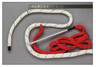
**2.5** Tape the fid to the bitter end of the core.
