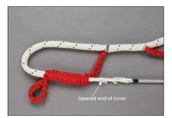
**3.7** Pull the fid out of the core exposing the entire fid and as much of the cover tail as possible. This will require bunching up the core back toward Core Mark 2.
