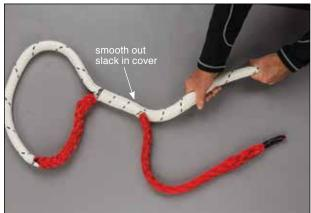
**4.2** Working from the standing part of the rope attached to the anchor point, milk or smooth out any slack in the cover towards the base of the eye. Continue to alternate between Step 4.1 and 4.2 until all slack is removed from the cover and the exposed core has been completely buried in the cover in the eye.
