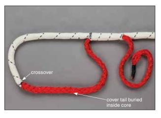
**3.8** Remove the fid and tape from the end of the cover. Pull the ends of both the core and cover until the marks on the cover and core are adjacent to each other. This is the crossover. Keep the marks tightly together for the remainder of the splice procedure.
