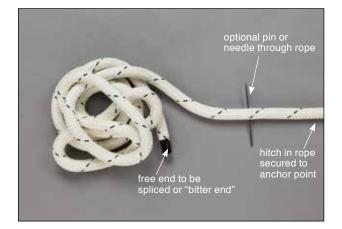
**1.1** Secure the rope to a sturdy post or anchor point by tying a hitch type knot 7–10 fid lengths down from the free end of the rope (the bitter end). If possible, insert a large sewing needle or pin through the rope just in front of the knot to assist in holding the cover and core together.
