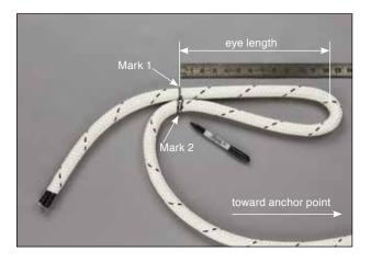
**Quality Check** Ensure accurate markings in Step 2. Inaccurate marks will directly affect the quality of the splice.
