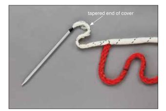
**3.4** Remove the fid from the bitter end of the core and tape it to the tapered bitter end of the cover.
