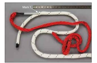
Mark 1 Mark 2 Mark 2 **2.6** Insert the fid into the cover at Mark I toward Mark 2.
