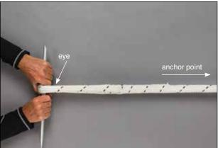
**4.6** To finish the splice, hold the top of the eye and pull against the anchor point. This will assist in removing any remaining slack in the rope and burying the exposed core in the eye. Cover slack can also be removed by milking the cover back towards the eye from the anchor point while keeping the rope under some slight tension.
