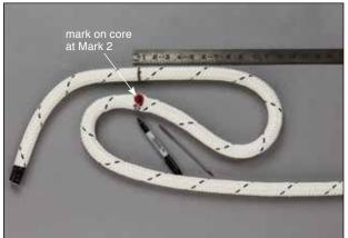
**2.2** Use a large needle, fid or similar tool to separate the cover yarns at Mark 2, exposing the core. Make a mark on the exposed core with the marker pen. This is Core Mark 1.
