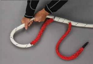
**3.9** Starting at the crossover, milk or smooth out any excess slack in the exposed core to bury the tapered cover tail. Then smooth out the cover braid from the crossover back to the point where the core tail exits from the cover.
