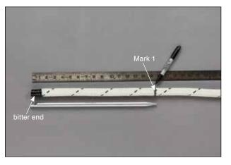
**1.2** Lay the rope out in a straight line from the anchor point to the free or bitter end. Using the fid chart, determine the appropriate fid length based on the rope diameter or circumference. Measure a distance equal to the fid length from the bitter end of the rope towards the anchor point and make a mark around the circumference of the rope (Mark I).
