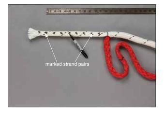
**3.1** Remove any tape around the bitter end of the cover. Working from Mark 1 on the cover count 5 picks (strand pairs) toward the bitter end of the rope and mark the 5th pair to form a V shaped mark on the cover. Then count down 4 picks and mark the 4th pair. Alternate counting and marking the 5th and then 4th pick (strand pair) until you reach the end of the rope.
