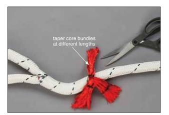
**4.4** Pull the core tail out from the cover about 1/3rd of a fid length and cut off the excess core tail at the mark that was just made. Then taper the exposed end of the core.
