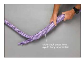
**4.4** Working from the base of the eye smooth out the bunched up rope away from the eye to bury the tapered bitter end back inside the body of the rope.
