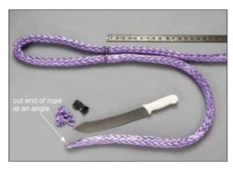
**3.1** Remove any tape from the bitter end of the rope and then cut the end of the rope at an angle.
