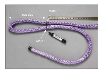
**2.1** Using Mark 1 as a reference point, form an eye in the bitter end of the rope. When the proper size of eye has been determined make a mark on the rope directly opposite Mark 1. This is Mark 2.
