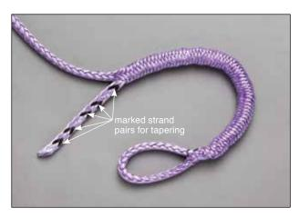
**4.1** Working from the bitter end, count 3 picks (strand pairs) away from the end and mark the 3rd pair to form a V shaped mark on the rope. Then count 2 more picks up the rope and mark the 2nd pair. Alternate counting and marking the 3rd and then 2nd picks for a total of five marked pairs, about 1 fid away from the bitter end (this forms a pattern of unmarked picks of 2-1-2-1-2 between marks).
