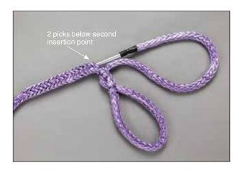
**3.7** At a point 2 picks below the last extraction point, insert the fid into the center of the rope and push it down the rope for a distance of 2-1/2 fids for Type 1 rope and 3-1/2 fids for Type 2 rope. Bring the tip of the fid out of the body of the rope at this point.
