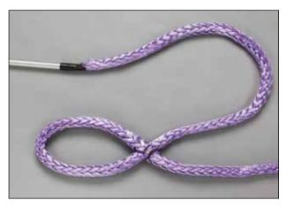
**3.4** Pull the fid and bitter end through until Mark 1 is buried inside the rope.
