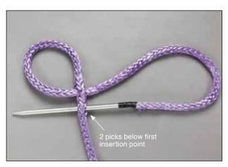
**3.5** Insert the fid through the rope at a point that is 2 picks below the first insertion point.
