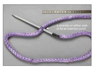
**3.3** Insert the fid directly through the body of the rope at Mark 2. The fid should be inserted between strands.
