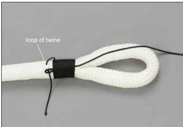
**1.3** Insert the end of the twine through the exposed loop.
