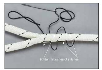
**1.5** Starting with the first series of stitches work out the slack in each loop until they are pulled flush against the surface of the rope. Do not pull the loops too tightly.
