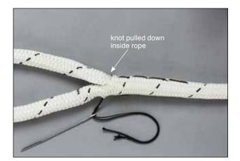
**1.9** Pull both ends of the twine completely through the rope. Pull on the ends to bury the knot into the body of the rope.
