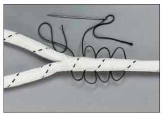
**1.4** Continue to stitch 3 more loops working back up the splice towards the base of the eye. Each loop should enter and exit the rope at the same point as the first series of stitches. When completed the needle and one end of twine will be on the same side of the rope as the other end of twine.
