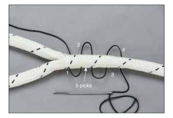
**1.2** Continue to stitch a total of 4 loops down the length of the splice following the same line of picks on each side of the rope. Each stitch should be 5 picks down from the point where the previous stitch comes out of the braid. This completes the first series of stitches. Do not pull the loops tight.
