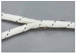
**1.10** Cut the excess ends of the twine close to the rope's surface.
