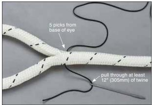
**1.1** Thread the needle with the twine and insert the needle directly through the rope at a point 5 picks below the base of the eye. When inserting the needle and pulling it out the other side of the rope make sure to go between strands, not through them. Pull through at least 12 inches (305mm) of twine when making the first stitch.
