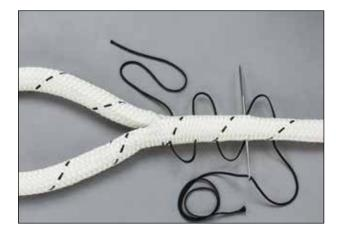
**1.3** For the second series of stitches, insert the needle back into the rope at the point where the last stitch on the same side is located and out on the opposite side of the rope where the previous stitch is located.
