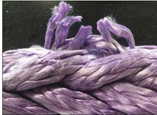
Visual inspection of interior yarns shows three fully cut yarns.
