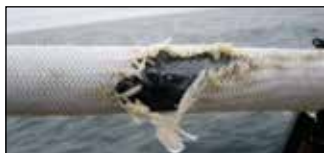
Fish bite pierced outer layer, but did not penetrate the aramid armor (photo courtesy Woods Hole Oceanographic Institute)
