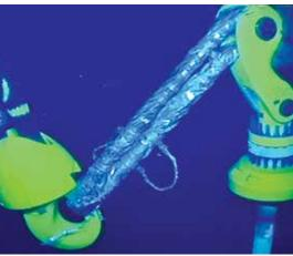
During the last decade, high-performance synthetic fiber lifting slings have been providing compelling improvements to operational efficiency and workforce safety over traditional steel wire rope slings. Both heavy equipment, and operations, benefit from advantages of synthetic fiber slings.
