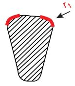
A DIN hook has an inconstant (not smooth) bearing profile in which the smallest radii in the profile must be taken into consideration when calculating the MBL or bending loss in a sling.
