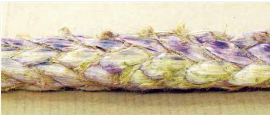
Example of burned and partially melted fiber
