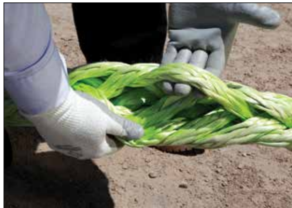
The rope can be inspected for internal wear / damage with the construction opened.
