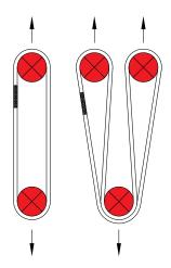
Represents a contact surface with a D:d ratio of one or greater. Refer to the Efficiency Table for deductions as needed.
