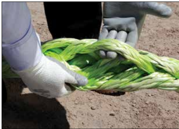
The rope sling can be inspected for internal wear / damage with the construction opened.
