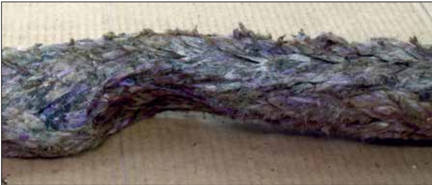
Example of burned and excessively melted fiber
