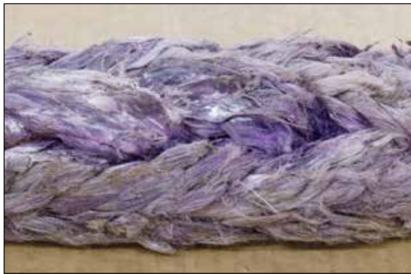
Glossy or glazed areas, fused or melted strands are signs of heat damage.
