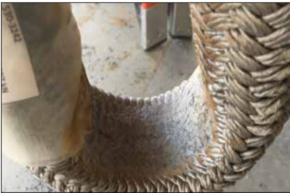
This is fiber compression. If the strands can be separated by flexing the rope, it is not heat damage.
